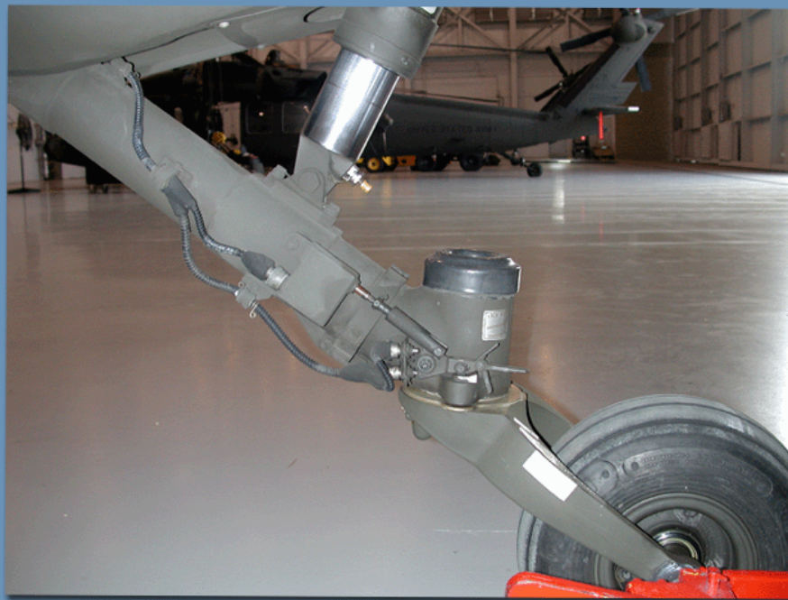
Frame #0275 (Tail Landing Gear Lock Actuator Location)
