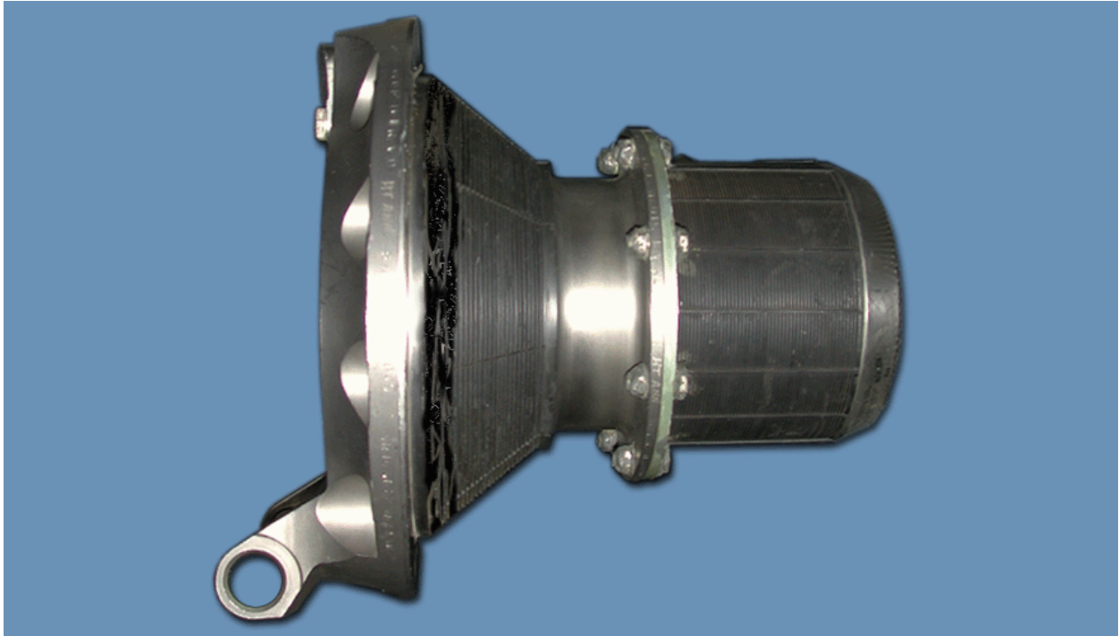
Frame #0245 (Elastomeric Bearing Extrusion)
