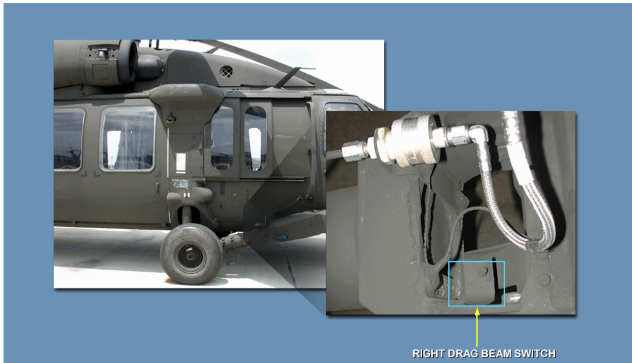
Frame #1012 (Right Drag Beam Switch)
