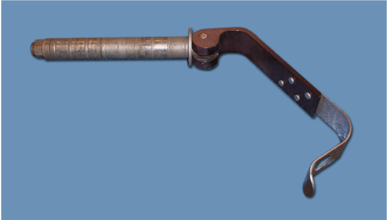
Frame #0610 (Main Rotor Blade Expandable Pin)
