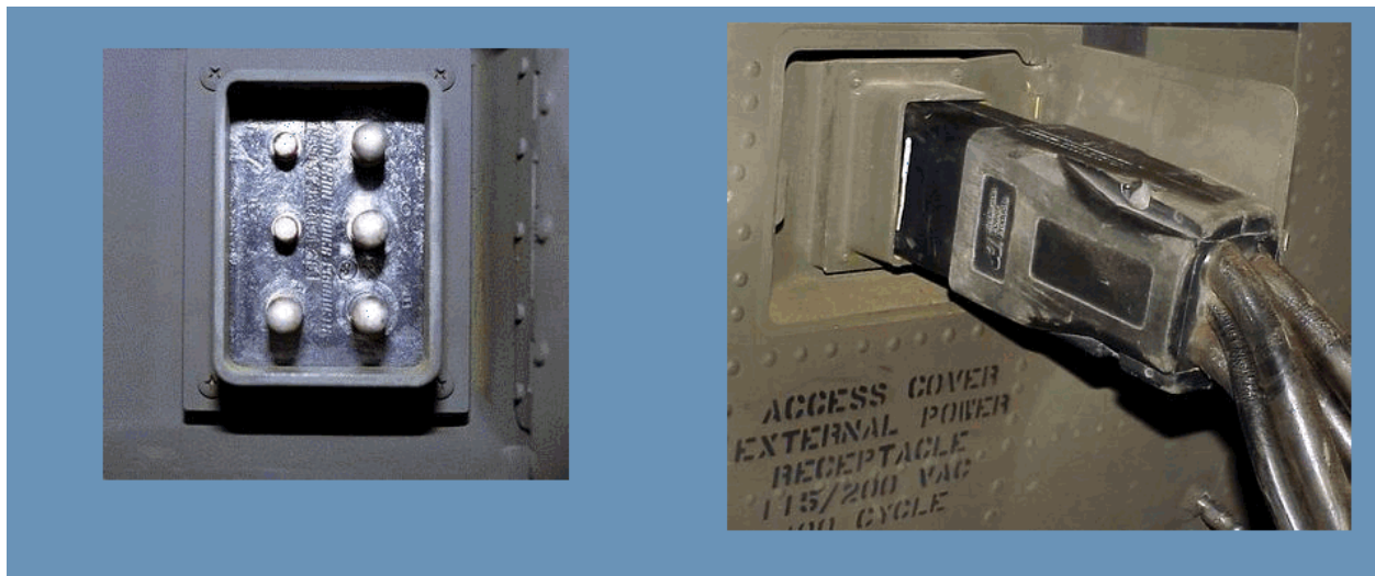
Frame #1065 (External Power Receptacle)
