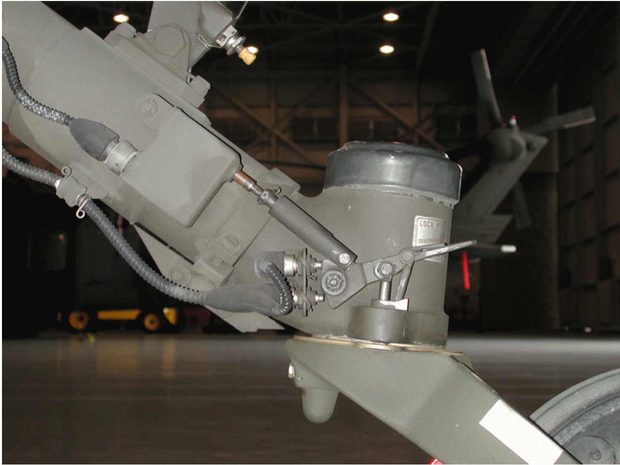
Frame #0280 (Tail Landing Gear Manual Release Lever)
