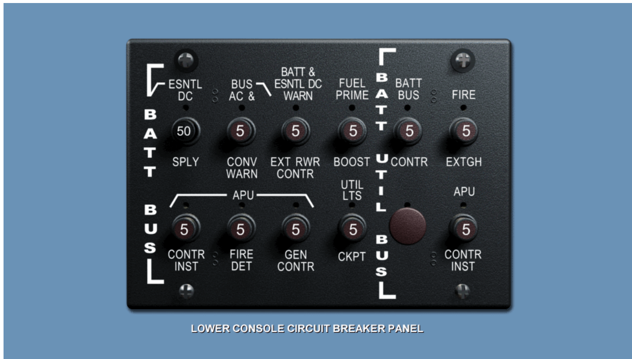
Frame #2083 (Lower Console Circuit Breaker Panel)
