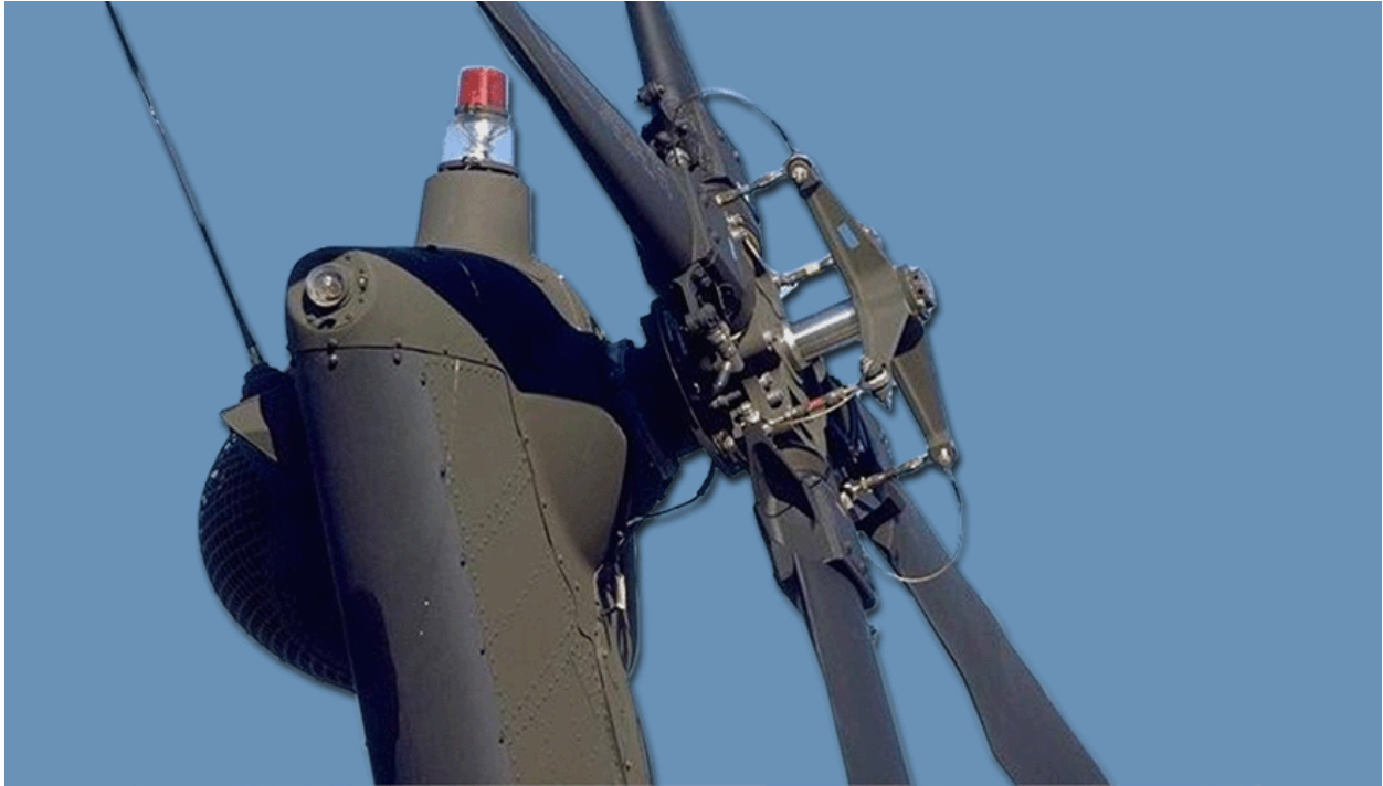
Frame #1065 (Pitch Control Rod Bonding Jumper)
